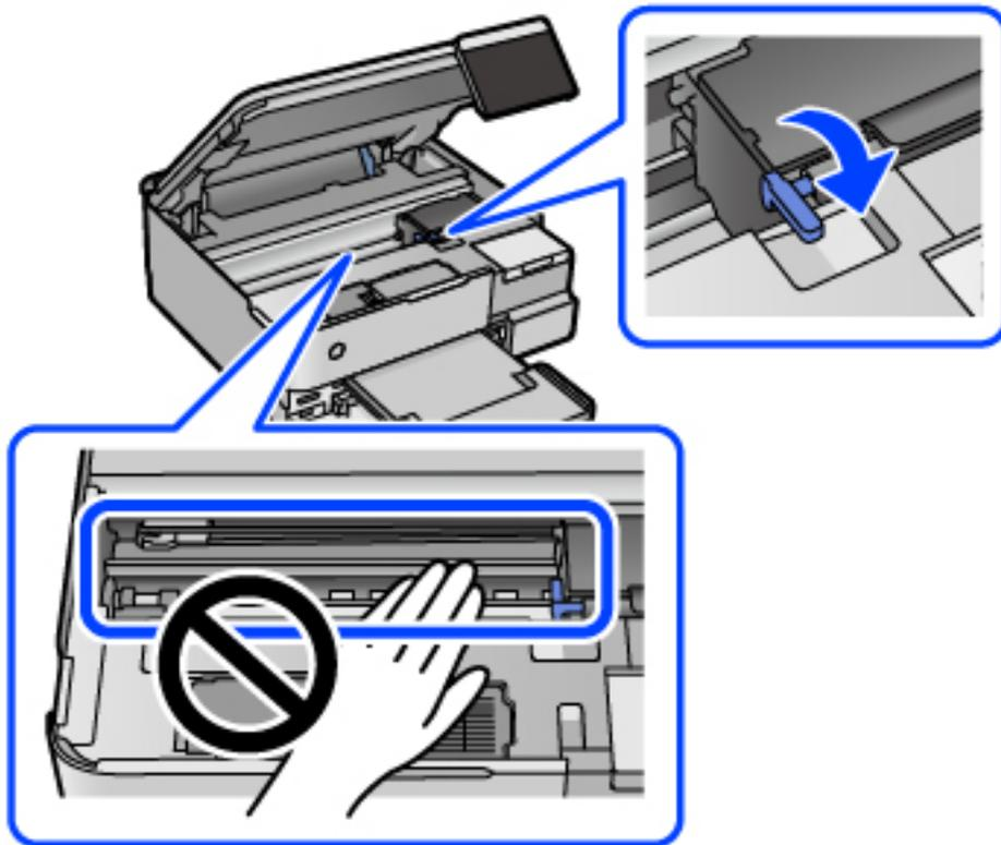
8. Secure the print head to the case with tape.
