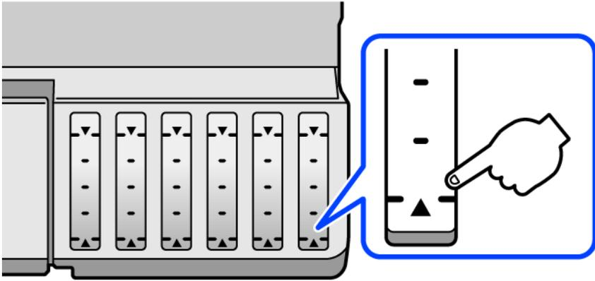
The diagram shows a side view of the printer's ink tanks. A blue callout box highlights one of the tanks, showing a vertical level indicator with two horizontal lines. A hand is pointing to the lower line, indicating the minimum ink level.
